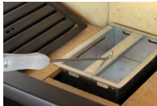
Ash pan removal from above.
