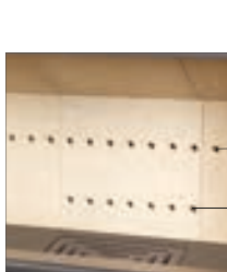
8 Tertiary or safety air. 9 Preheated primary air.
