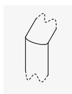
Finished flue corner piece
